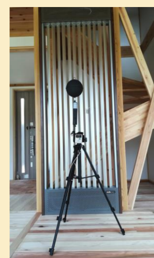
Figure 1 the model house in Nara Figure 2 radiation panel and PMV meter Figure 3 the condition of experiment (left: dehumidification amount, right: room temperature)
