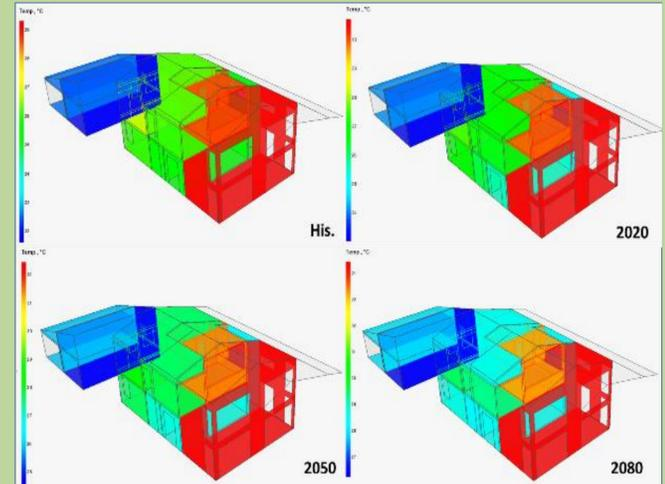
Figure 5: Mean air temperature in the zone at the time of maximal heat removed under different climate files
